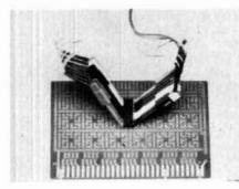
Incorporated into the design is a one-piece, gold-plated beryllium copper conductor and hook for assured signal accuracy, qualified to MIL-G-45204. The P-25 permits connection to 0.025-inch square or 0.030-inch round push-on umpers and is designed for connection directly to a single leg of a DIP or other components which have a maximum diameter of 0.025 inch.
